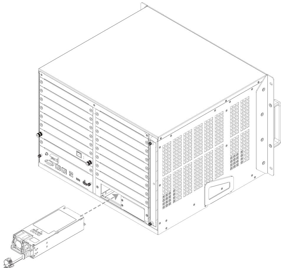
4. Plug the power cord into the 3 prong socket of the power module.
