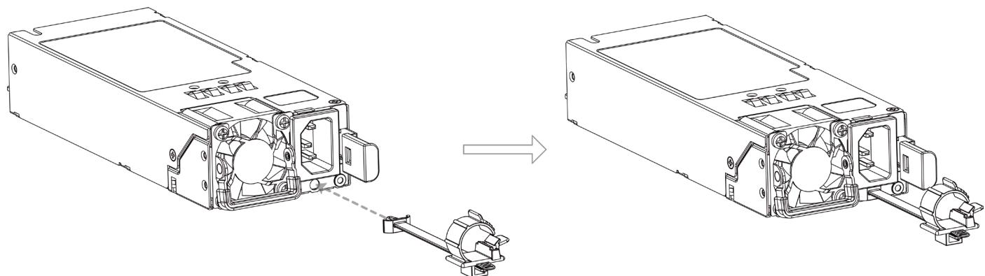
2. Install the power module to a power slot on the rear side of the VW3620 video wall processor:
