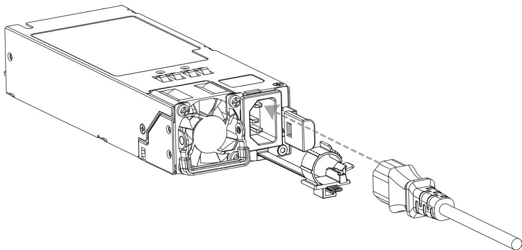
5. Secure the power cord by moving the buckle to the strain relief side of the power cord.
